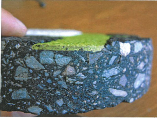
Dura Therm cross-section. Dura Therm is an imbedded thermoplastic product.
