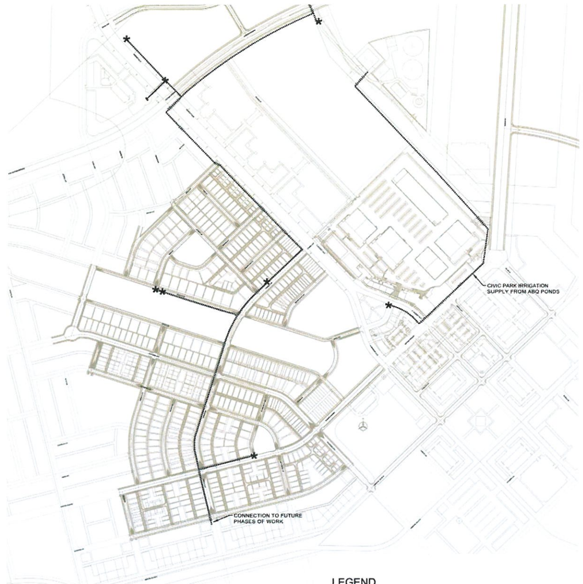
Re-use 'purple pipe' system
